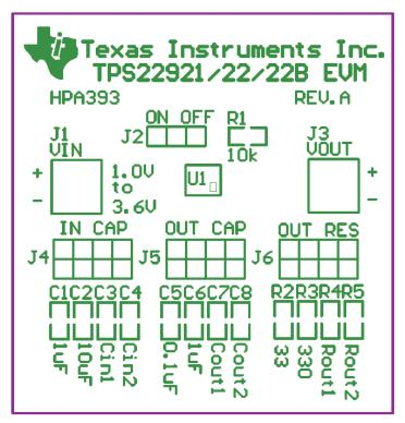
Figure 3-1. TPS22921/22/22B EVM Component Placement
